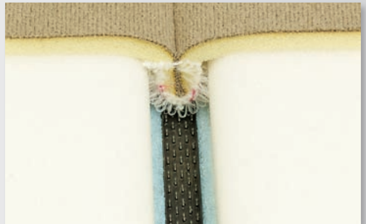
A gasketed HF3 12 fastener in the foam bun engages the VELCRO® Brand Loop Auto sewn onto the trim cover. The loop fits snugly in the trench to minimize seat trim line variation.
